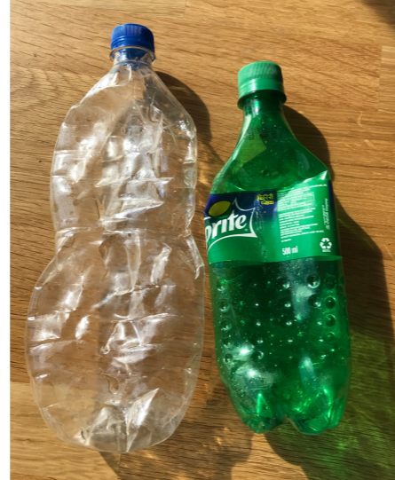
Water bottle left (thin plastic, produced in the region) and Sprite bottle (heavier plastic - imported)
