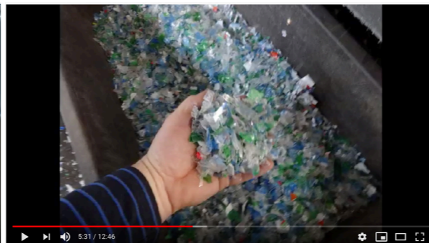
Stage 2: Bottles shredded into chips
