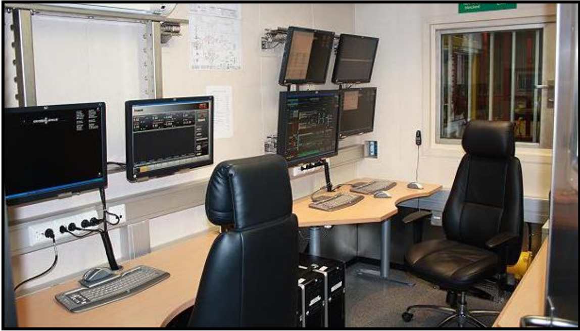
Figure 8: An example of a control cabin for MPD operation (with permission from Halliburton AS).
