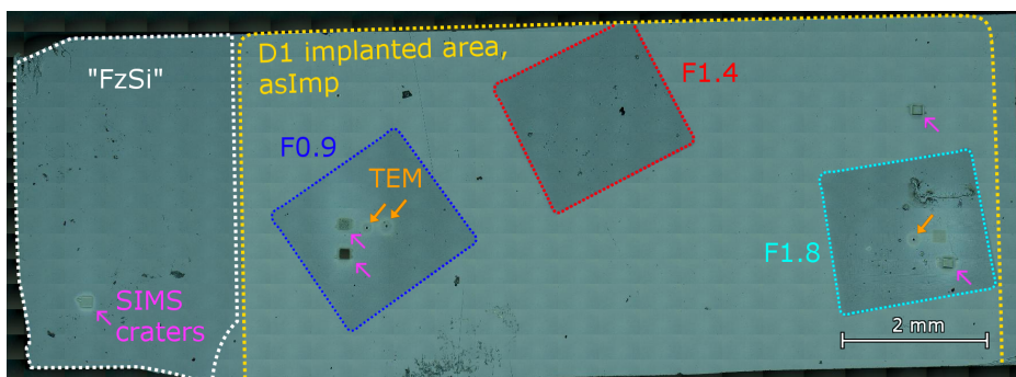
Figure 4.1: Overview image for wafer piece W-D1 from optical stitching. The area with 1 at.% W implantation is indicated with a yellow border and labelled "asImp". The "FzSi" area is indicated with a white border. The PLM spots of fluences 0.9 \text{ J}/\text{cm}^2 , 1.4 \text{ J}/\text{cm}^2 , and 1.8 \text{ J}/\text{cm}^2 are indicated in their respective colours of blue, red, and cyan, and labelled F0.9, F1.4, and F1.8. Purple arrows indicate SIMS sputter craters, while orange ones denote TEM wells.
