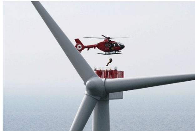
Figure 1.8: Helicopter used for maintenance tasks at an offshore wind turbine. Photo: Bond Aviation Services
