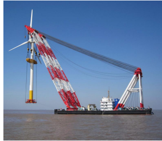
(a) An example of a crane vessel. Photo: classifieds.justlanded.com
