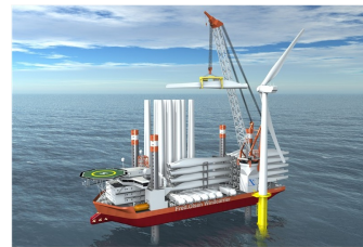
(c) The Windcarrier jack-up vessel by Fred. Olsen. Photo: Windcarrier.com
