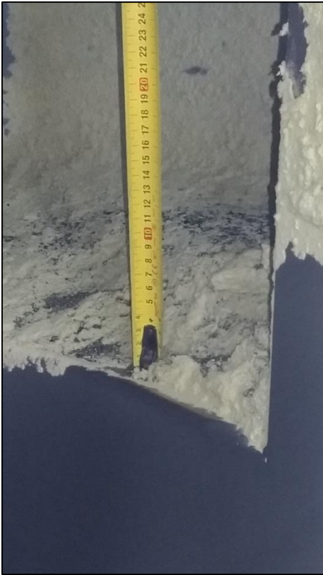
Figur B.9: Mengde groing
