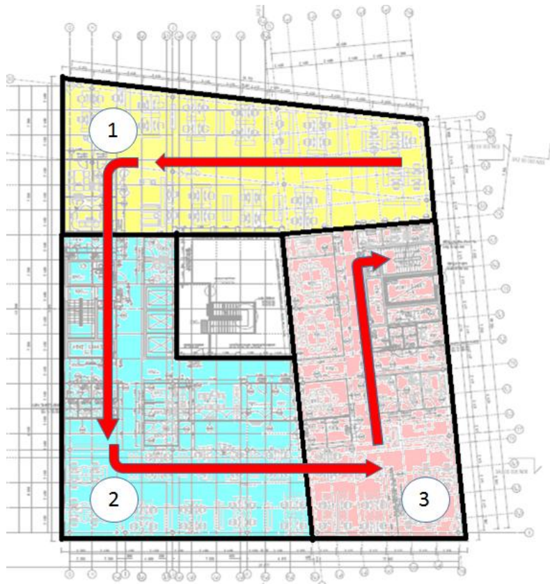
Figure 28 - New LBS within the floors and roof with suggested path to follow
