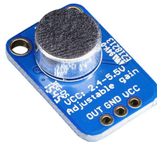
Figure 2.5: MAX4466 microphone amplifier [12]
