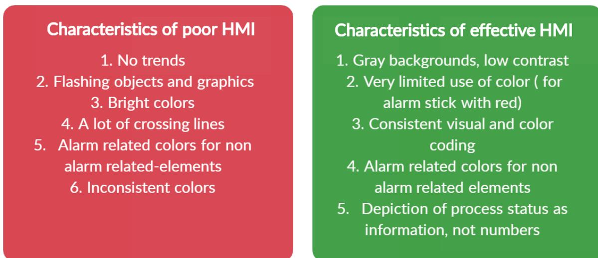
Figure 38: HMI Characteristics
