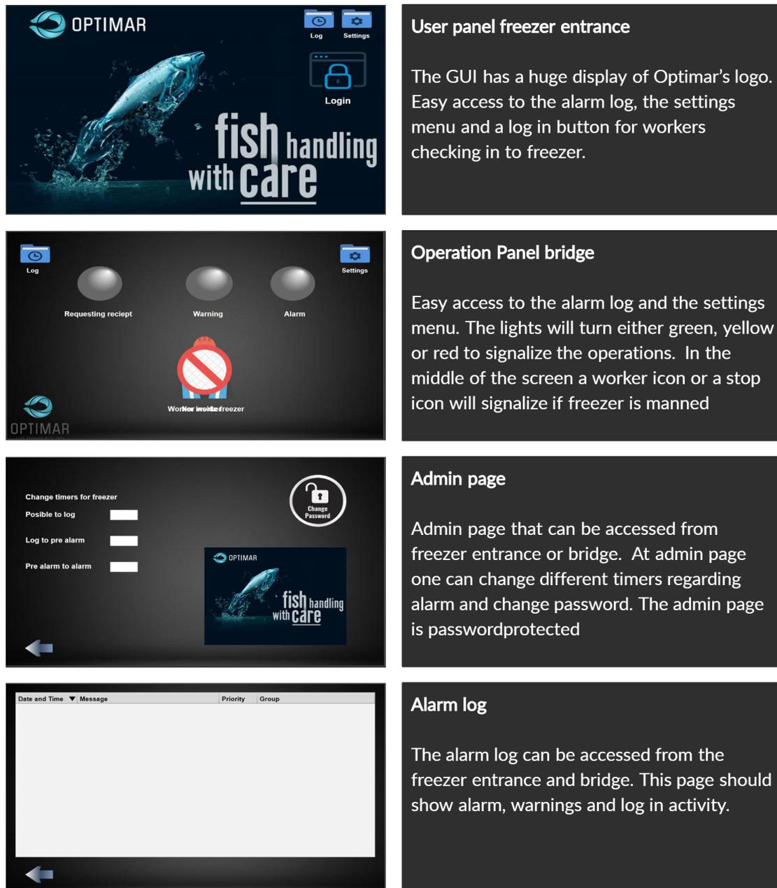
Figure 39: HMI test design 1
