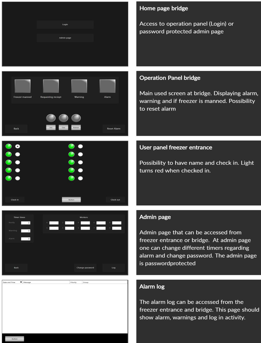
Figure 40: HMI test design 2
