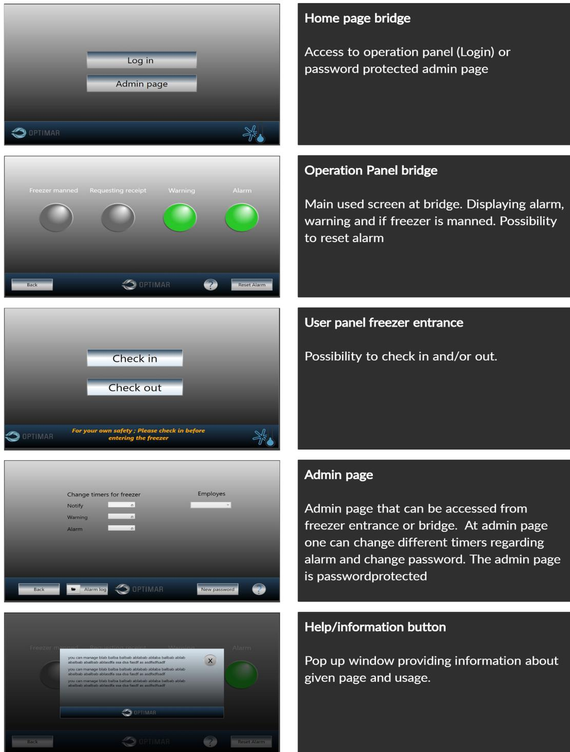
Figure 41: HMI test design 3
