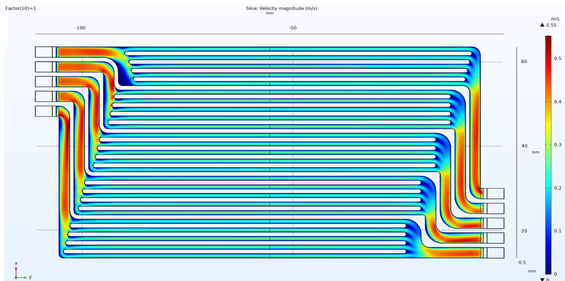
Figure 3.1.11: Velocity field of the channels in the final design at 50g/min per channel. Dimension specified in figure A.6.1
