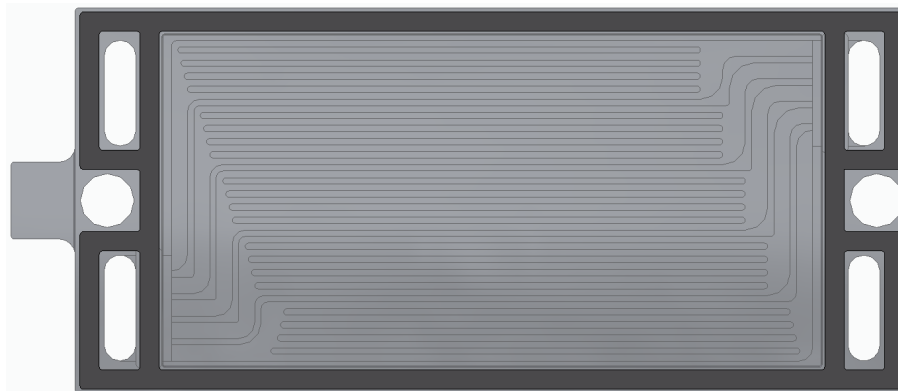
Figure 2.2.10: Illustration of the gasket assembled on a bipolar plate. Dimensions specified in appendix A.5.
