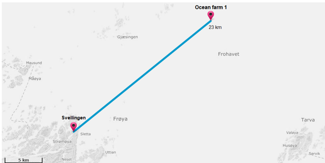
Figure 7.4: Svellingen at Frøya, approximately 23 km from Ocean Farm 1, have sufficient capacity in the existing grid of 11 kV to cover the power demand of Ocean Farm 1. The blue line represents the length of the subsea cable. The length does not include the depth of the sea or possible obstacles on the sea bed.
