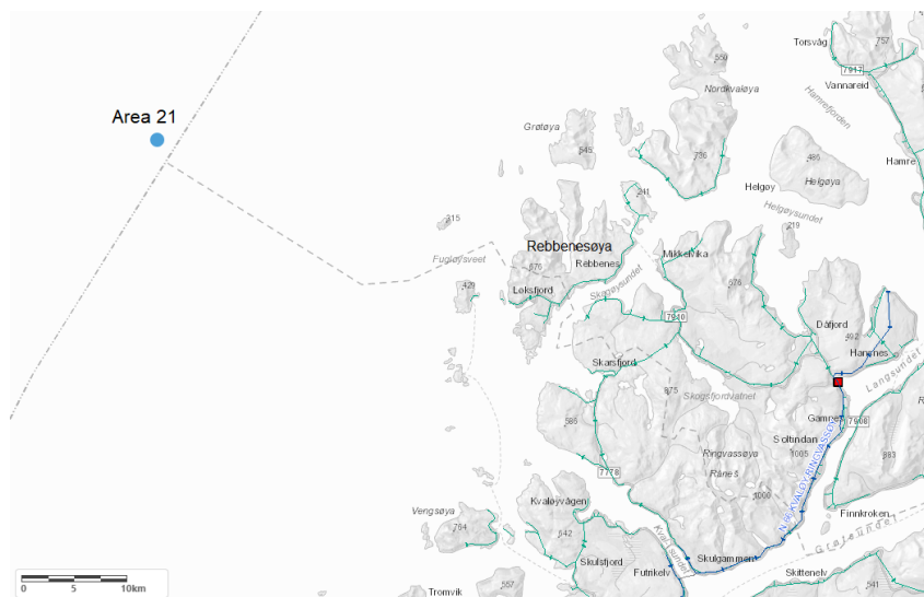
Figure 6.10: The closest electricity grid to area 21 is the 22 kV grid at Rebbenesøya.[116]
