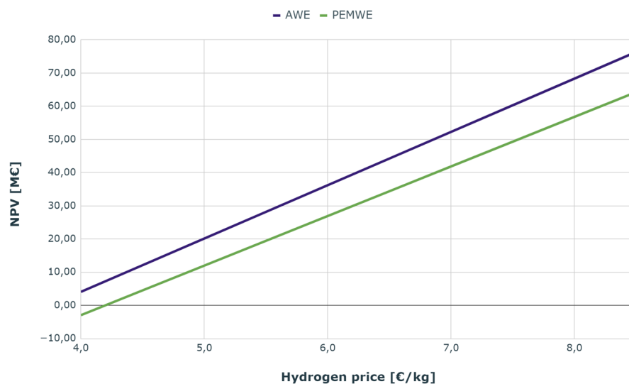
Figure 37: NPV analysis for an array of hydrogen prices, using all available power.
