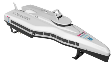
(c) ZeFF (Zero emission Fast Ferry) will advantage from hydrofoil technology, and is planned to use about 265 kg of H 2 one way. [28]
