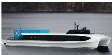
(a) Aero 42 H2, designed by the Brødrene Aa consortia. It is planned to use about 360 kg of H 2 one way. [23]
