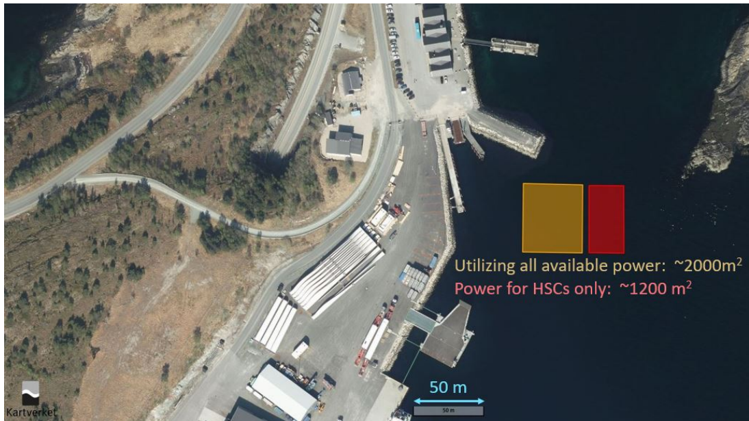
Figure 42: Total area footprint given by AWE, location Hitra Harbor. Based on a screenshot from Norgeskart made by Kartverket. [134]
