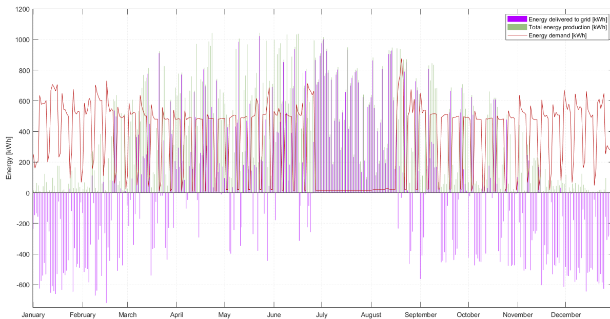
Figure 4.2: The Original scenario simulated with 959 m 2 of solar PV production for a year. Yellow represents total daily solar energy production, red represents total daily energy demand of the school and purple is the total daily energy delivered or taken from/to the grid.
