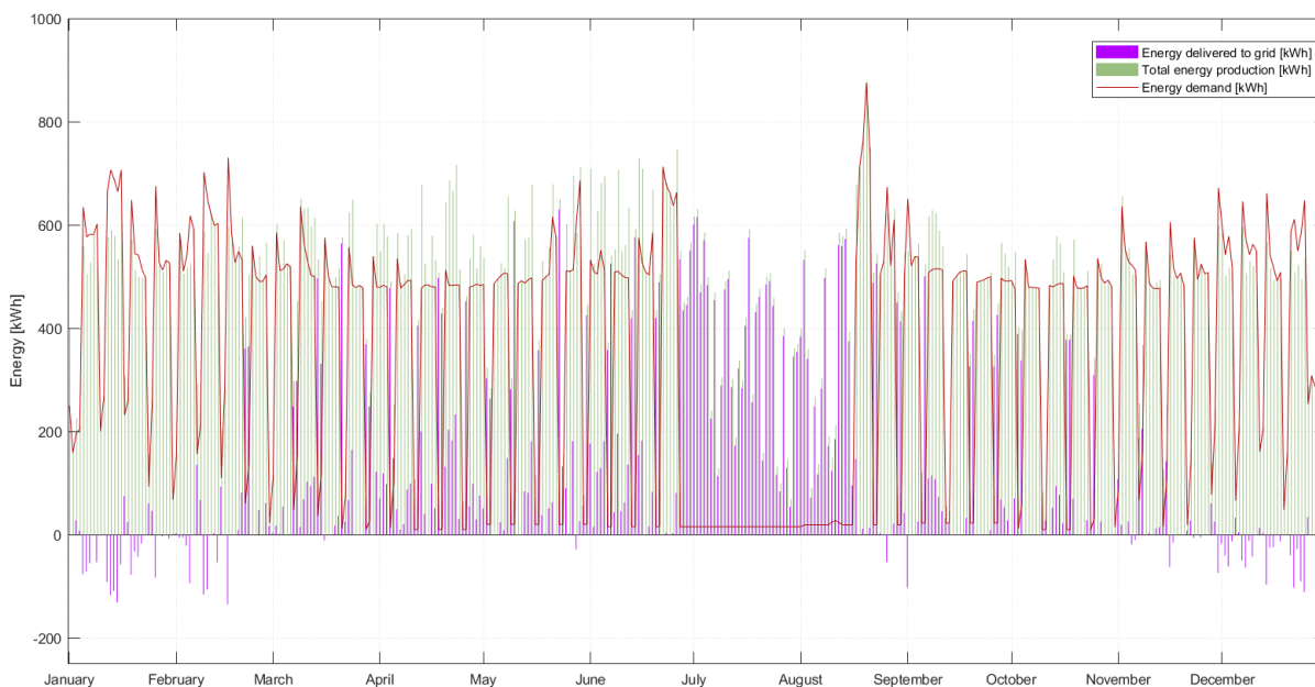
Figure 4.9: 2-A simulated with the hydropower plant, 600 m 2 and a 150 kWh battery for a year. Green represents daily total energy production, red represents daily total energy demand of the school and purple is the daily total energy delivered or taken from/to the grid.
