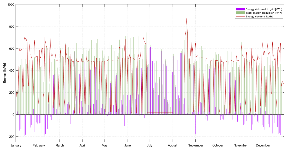
Figure 4.10: 2-B simulated with the hydropower plant, 600 m 2 and a 75 kWh battery for a year. Green represents daily total energy production, red represents daily total energy demand of the school and purple is the daily total energy delivered or taken from/to the grid
