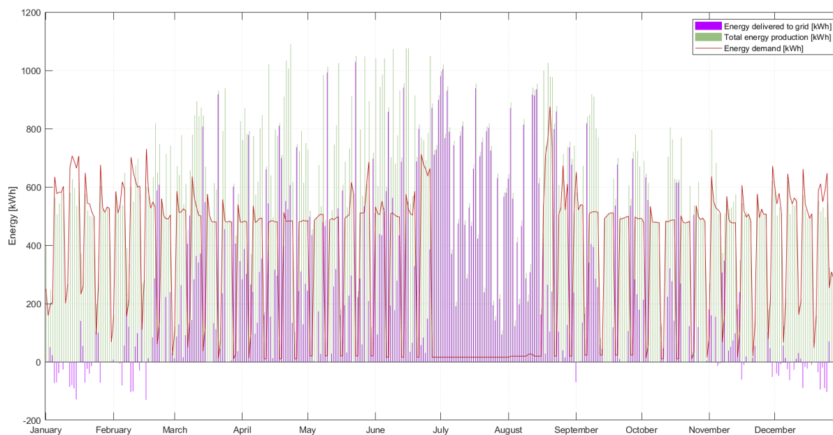
Figure 4.6: 1-A simulated with the hydropower plant, 959 m 2 of solar PV and a 150 kWh battery over a year. Green represents total daily energy production, red represents total daily energy demand of the school and purple is the energy total daily delivered or taken from/to the grid.
