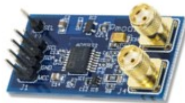
Figure 4. DigilentPmod IA AD5933 sensor (Source: < https://store.digilentinc.com/pmod-ia-impedance-analyzer/ >)
