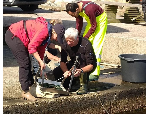
Figure 2.5: A Hydrobios™ dredge was used to sample bottom dwelling organisms. Photo Torkild Bakken
