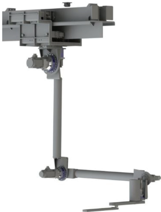
Fig. 5. A CAD model of robot 2, mounted on the horizontal linear axis.
