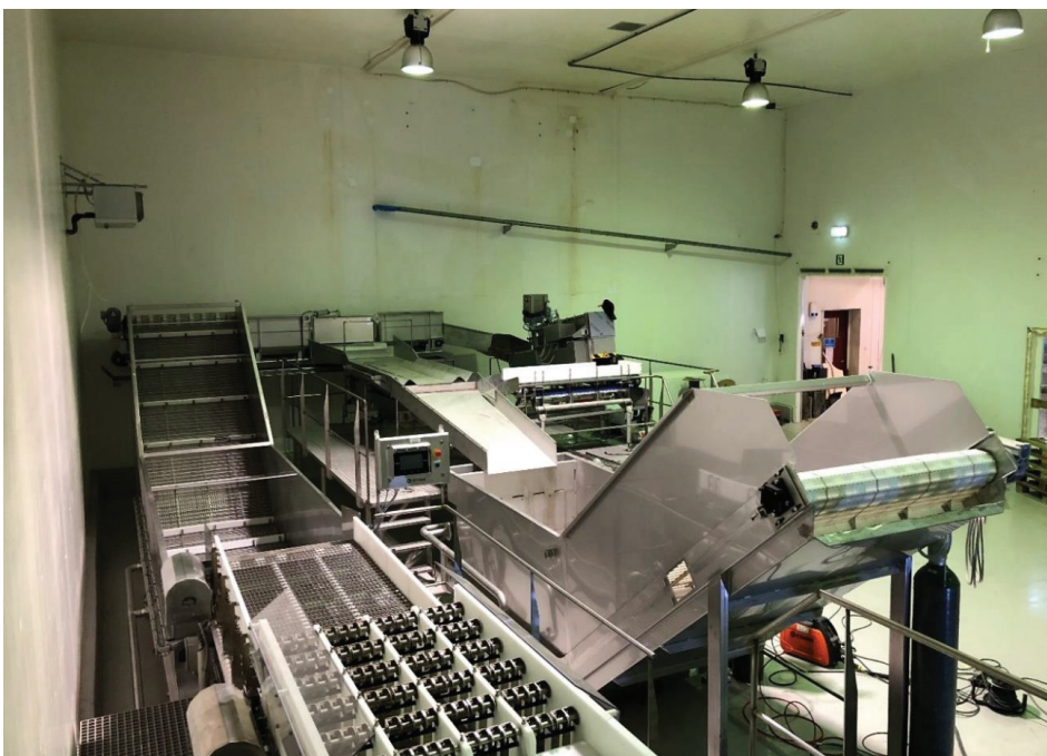
Figure A.9 Slaughter line at FPP 4. Consider the vastly different layout from previous pictures.
