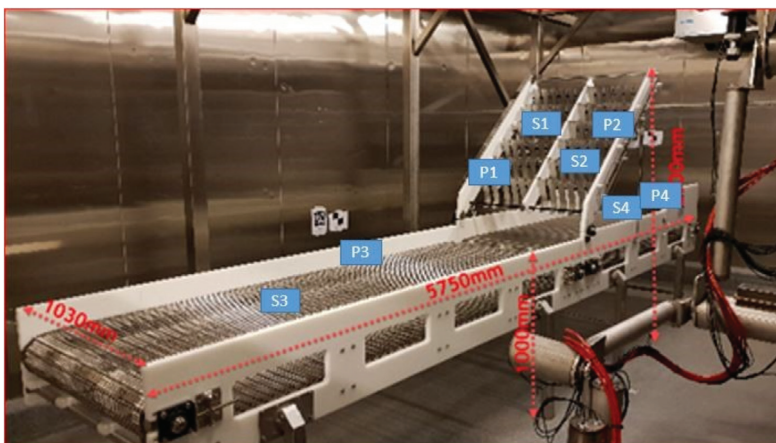
Fig. 12. Control points and dimensions of equipment in Experiment 2. The electric stunner in the cleaning position with the conveyor belt connected at the front. Sampling points for microbiological analysis in Experiment 2 are indicated as follows: S1 and S2 are steel lamellae on the electrical stunner; P1 and P2 are plastic walls inside the electrical stunner; S3 and S4 are steel cross-beams under the belt of the conveyor and the stunner, respectively. P3 and P4 are the inside plastic walls on the conveyor and the stunner, respectively. (Care was taken not to sample the same areas before and after cleaning).
