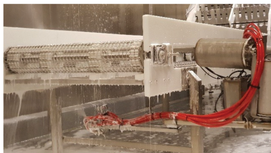
Fig. 17. Prototype 2 spraying soap.
