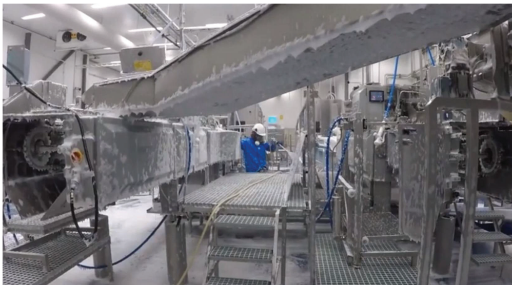
Figure 3.1 Environment of an FPP and the use of a manual cleaner during cleaning.
