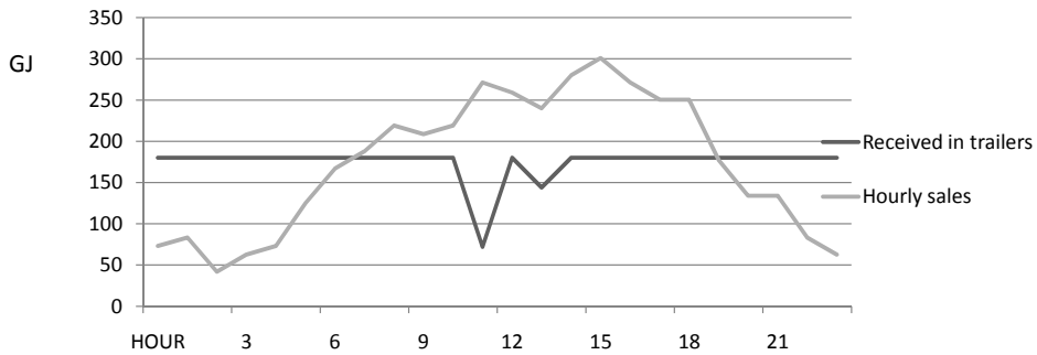
Figure 3.13: The storages make it possible for the trailers to have arrival rates that do not correspond directly to the short-term demand variation. Example is the supply from large scale reformer at 14 to region 4 in year 2048 in the high electricity price case.
