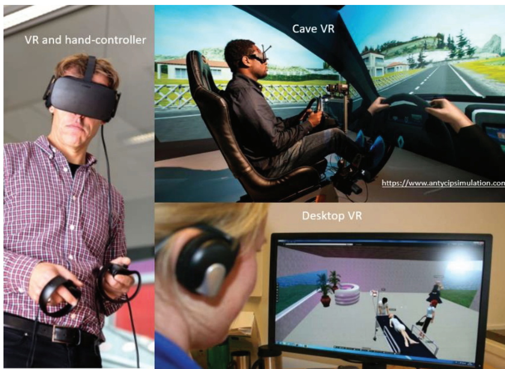
Figure 1. VR head mounted display and hand controllers, desktop VR and cave VR.
