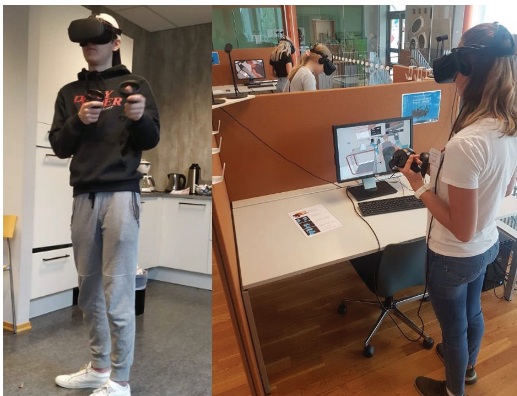
Figure 4. Oculus Quest (left) with no cable to a compute, and Oculus Rift (right).
