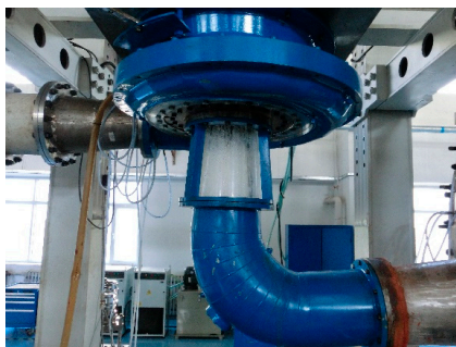
Figure 2. The pump-turbine model.
