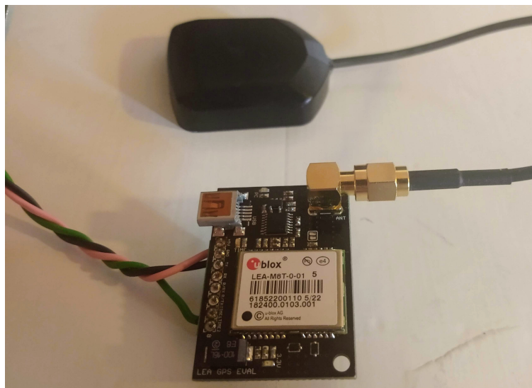
Figure 3.6: One of the GPS-units connected to antenna.
