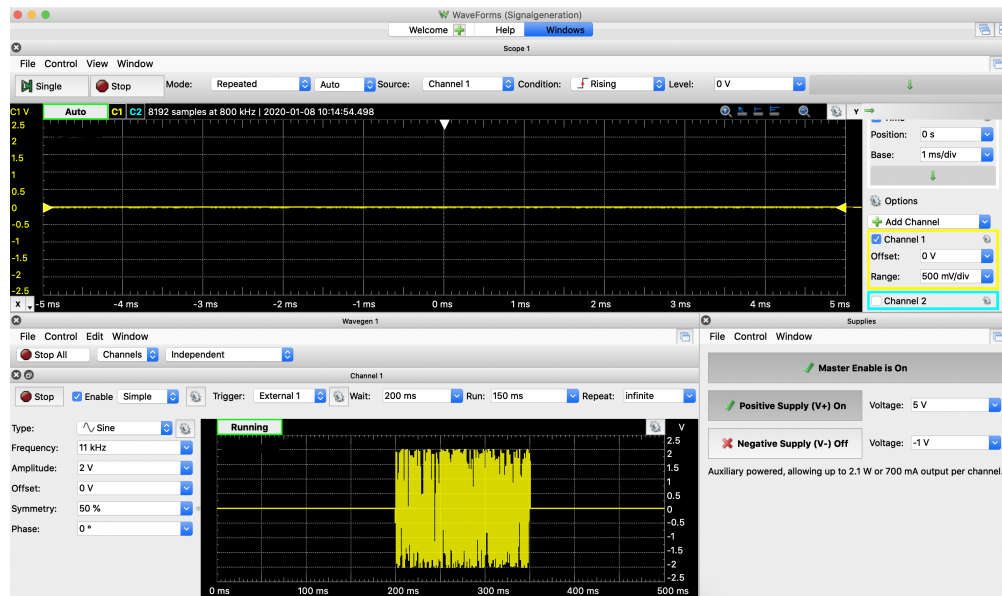
Figure 3.4: The oscilloscope interface while armed to generate pulse when triggered
