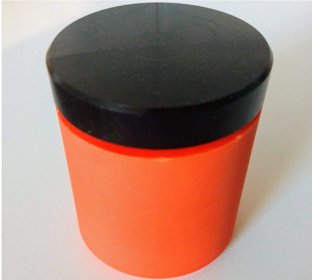
Figure 3.10: The mobile transducer with a epoxy layer and water tight lid.
