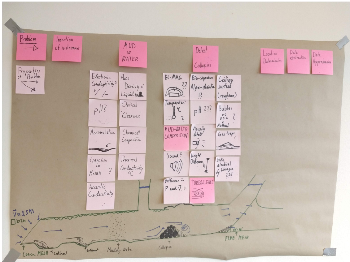
Figure 2.5: A rough sketch of Simsfossen, aspects of an inspection and their potential physical properties
