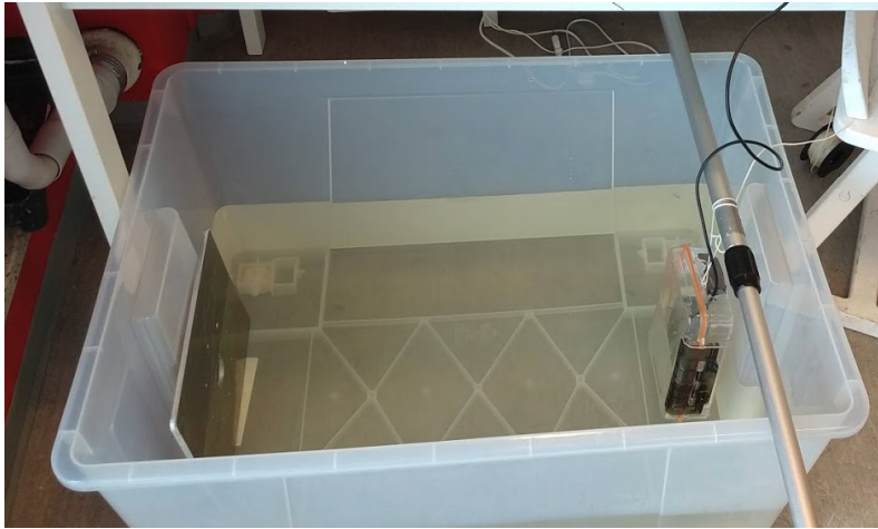
Figure 3.3: Test setup of the the radar sensor submerged in water.
