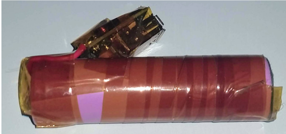
Figure 3.16: The battery used to power the sensor package with power.
