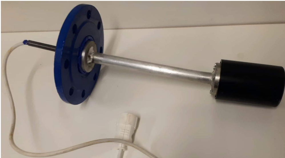
Figure 3.7: The final mechanical structure of the pinger.
