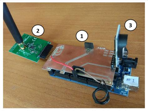
Fig. 2 Experimental node setup showcasing the baseboard, RF module, and other peripherals
