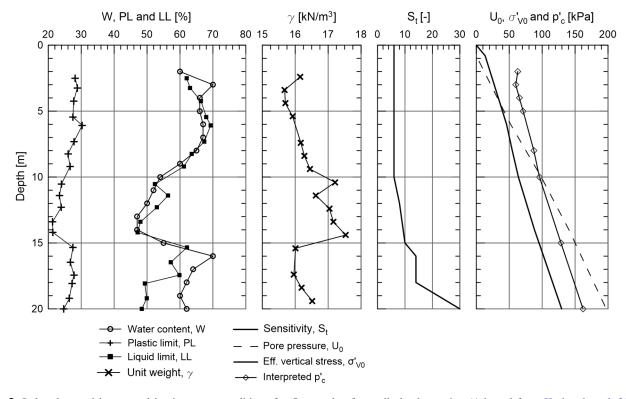
Fig. 3. Index data and interpreted in situ stress conditions for Onsøy clay from pile load test site. (Adapted from Karlsrud et al. 2014.)
