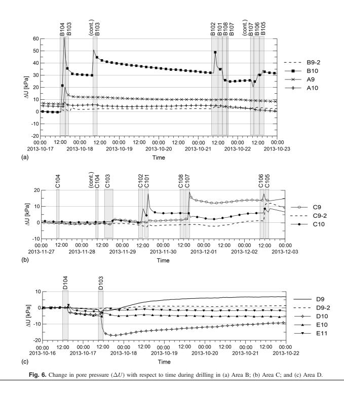
the pressure reduction in PZ D10, caused by suction in the clay above the cavity in the sand/moraine layer.
