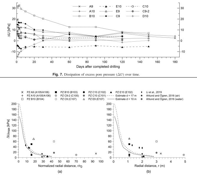
Fig. 8. Maximum change in pore pressure ( $\Delta U_{max}$ ) against (a) normalized radial distance; and (b) metric radial distance from anchors (casings).
