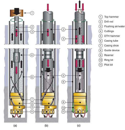
**Fig. 1.** Rotary percussive duplex drilling methods and drill bits used for overburden drilling: (a) top drive (top-hammer) eccentric; (b) DTH hammer eccentric; and (c) reverse circulation (RC) DTH hammer concentric.
