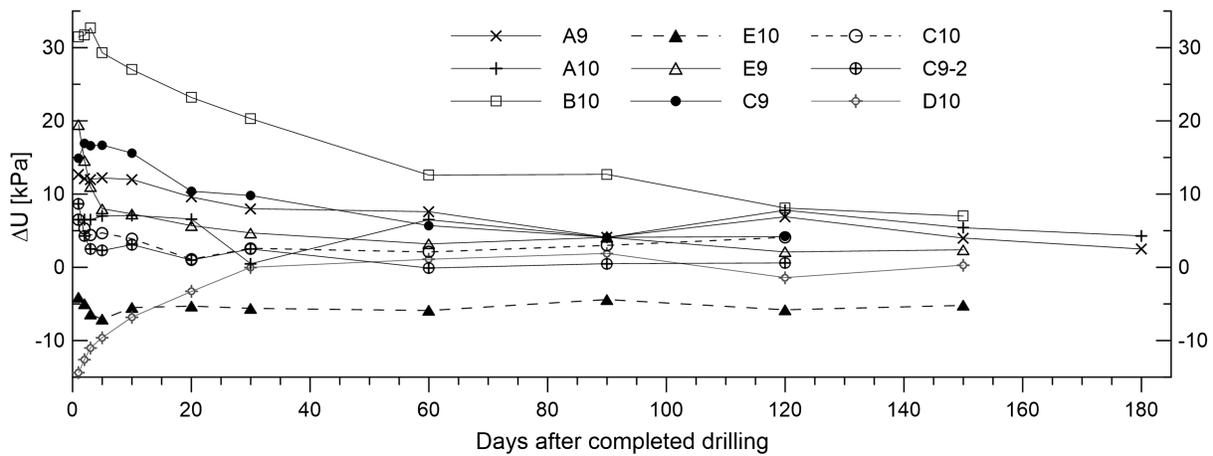
Fig. 7. Dissipation of excess pore pressure ( $\Delta U$ ) over time.
