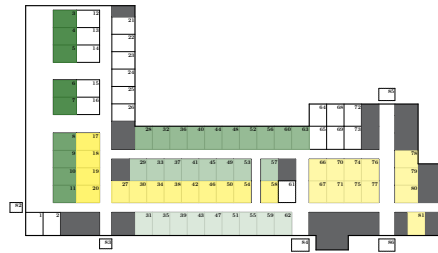
Figure D.6: Feasible locations for the storage rooms in green and the bathrooms in yellow. The different shades of each color indicate where the different storage rooms and bathrooms can be allocated.
