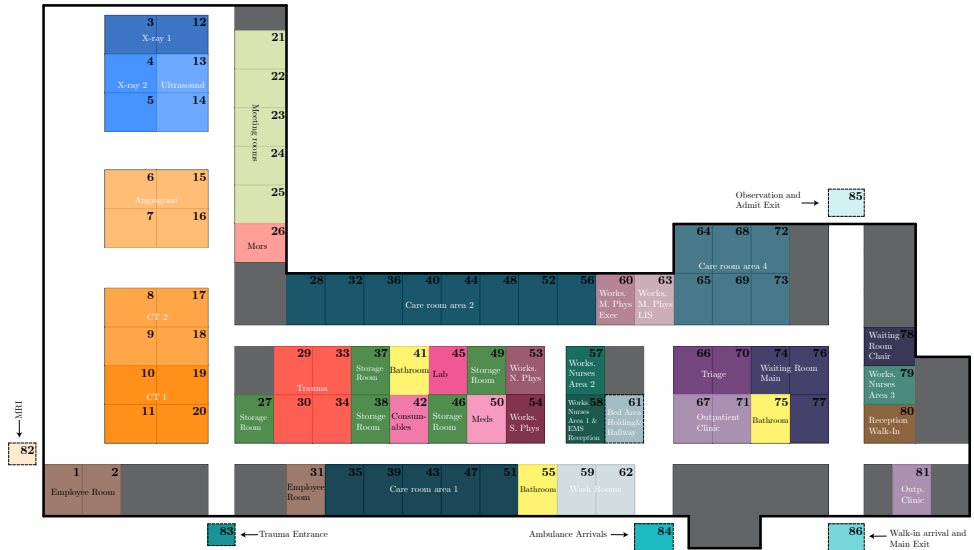
Figure 9.1: Today's layout of the Kalnes ED, presented in the grid used in the optimization model.
