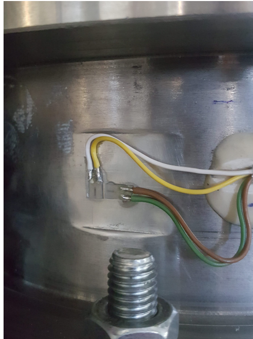
Figure 3.3: Flattened sections of the ATMD and the previous used semiconductor strain gauges.
