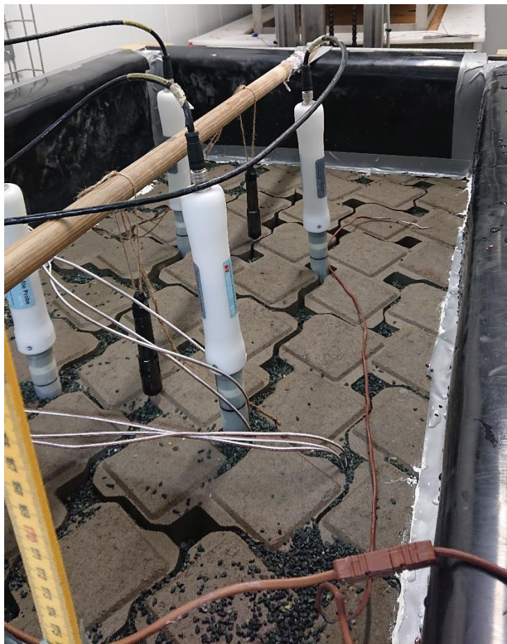
Figure 5: Picture showing how the joint material have been lifted from the slits during the first test Photo: Heidi Jensen
