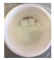
Figure 4.2.2: Image of the partially broken green body after sublimation of the ice in the initial freeze casting.
