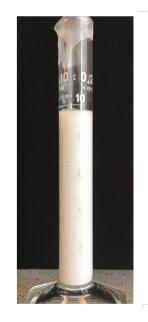
Figure 4.2.1: Image of the stable BCZT aqueous suspension from the sedimentation test, 5 hours after mixing, achieved by the addition of an ammonium polymethacrylate dispersant.
