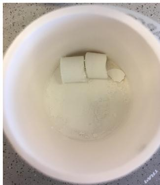
**Figure 4.2.2:** Image of the partially broken green body after sublimation of the ice in the initial freeze casting.
