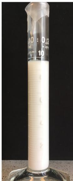
**Figure 4.2.1:** Image of the stable BCZT aqueous suspension from the sedimentation test, 5 hours after mixing, achieved by the addition of an ammonium polymethacrylate dispersant.
