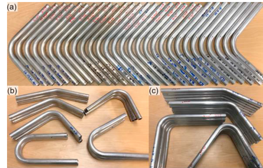
Fig. 4. Experimental bent tubes: (a) with different pre-NA time; (b) bent tube after SHT without aging; (c) as-received tubes with T4 temper.
