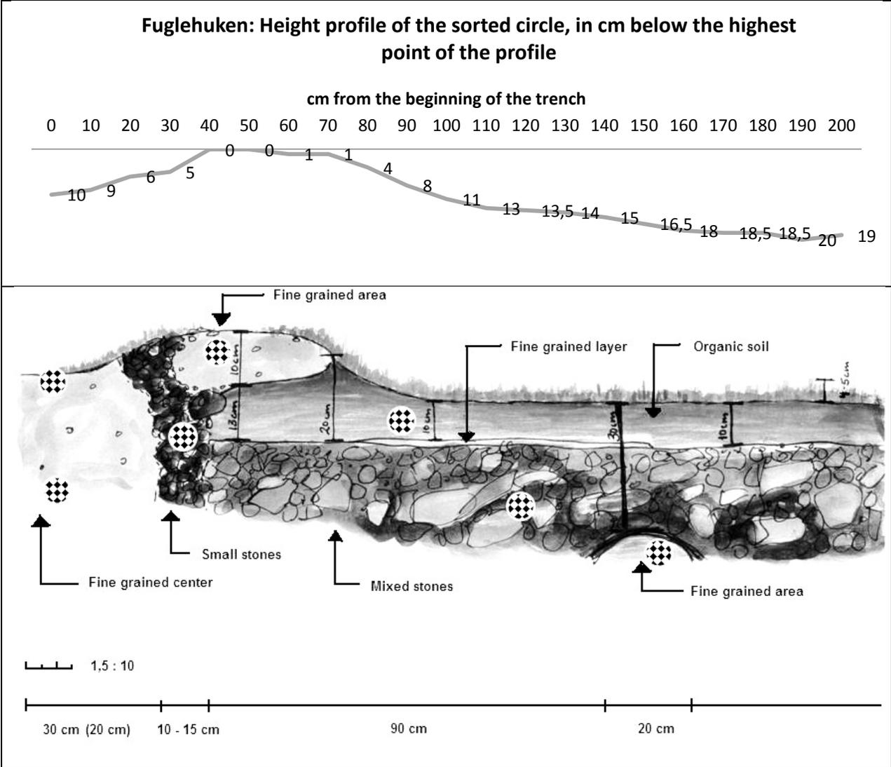
Figure 4: Schematics of the trench dug through a sorted circle. To the far left the center point of the circle is shown, following the trench dug through the border into the area outside the circle. Points in the profile marked with a checkered pattern show where soil was sampled. The line on top of the schematics shows the measured surface profile relative to the highest point of the border
