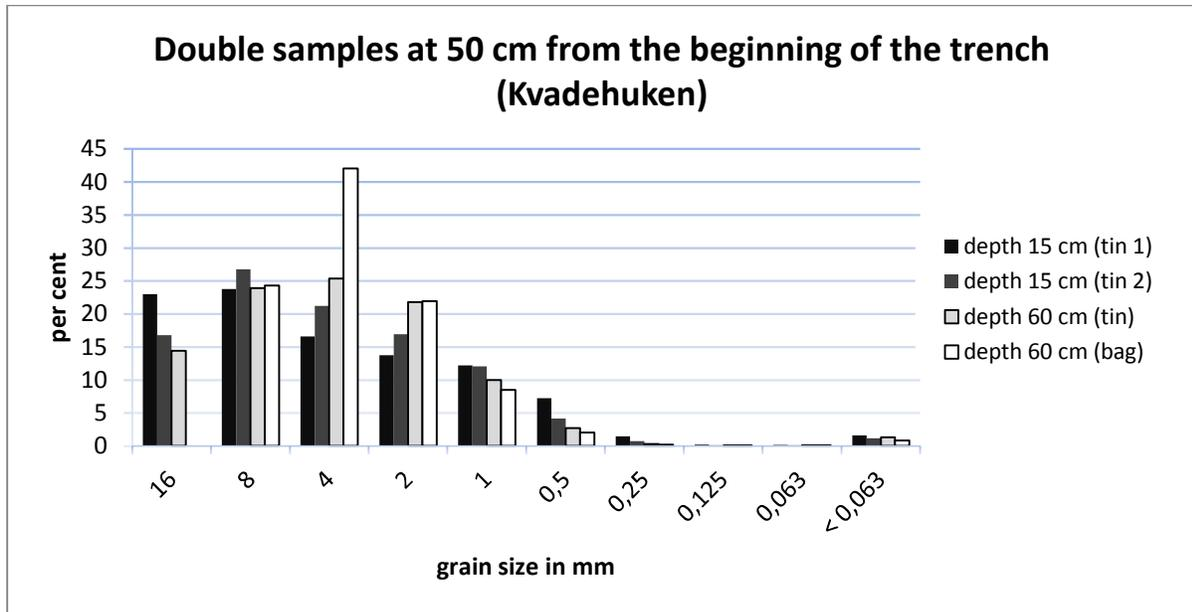
Figure 3: Grain size distribution from two sets of double samples taken at the same depth. Both sets are sampled from the coarse border, at 50 cm from the beginning of the trench dug through the sorted circle in Kvadehuken. -> why is there a sudden peak at 4mm instead of at 8mm?
