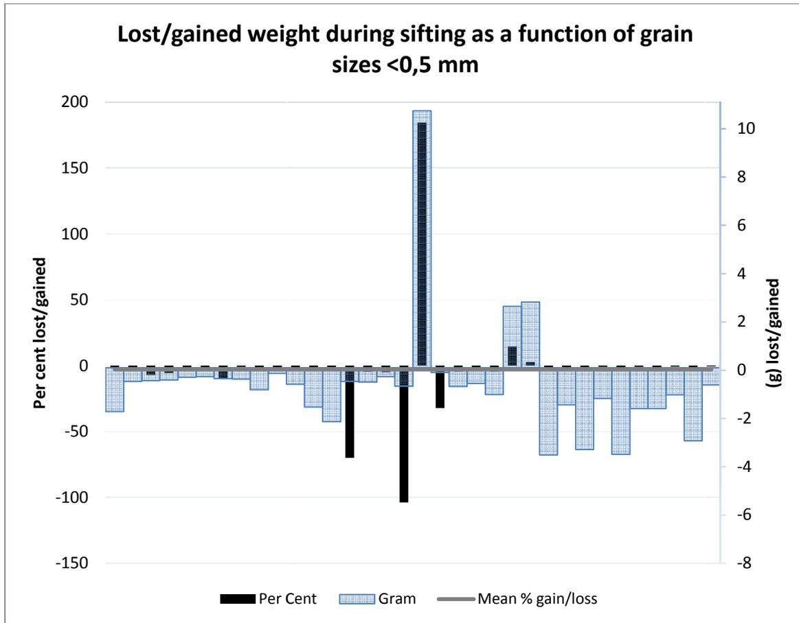
Figure 2: Per cent difference in mass before and after sifting of grain sizes smaller than 0,5 mm. The line indicates a loss of about 3 % from these smaller particle sizes. Samples presented here are from both Kvadehuken and Fuglehuken.
