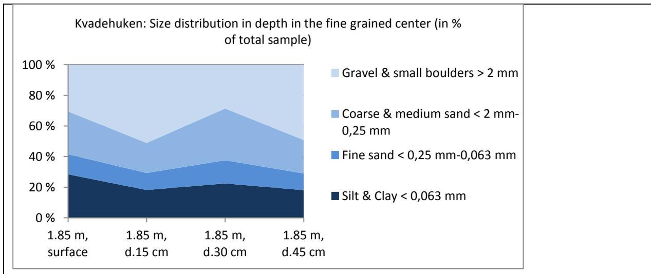
Figure 5: Kvadehuken: Size distribution at different points in the section, following the soil profile from the surface and down. The sizes of gravel, sand, slit and clay are shown in percentage of the total sample.
