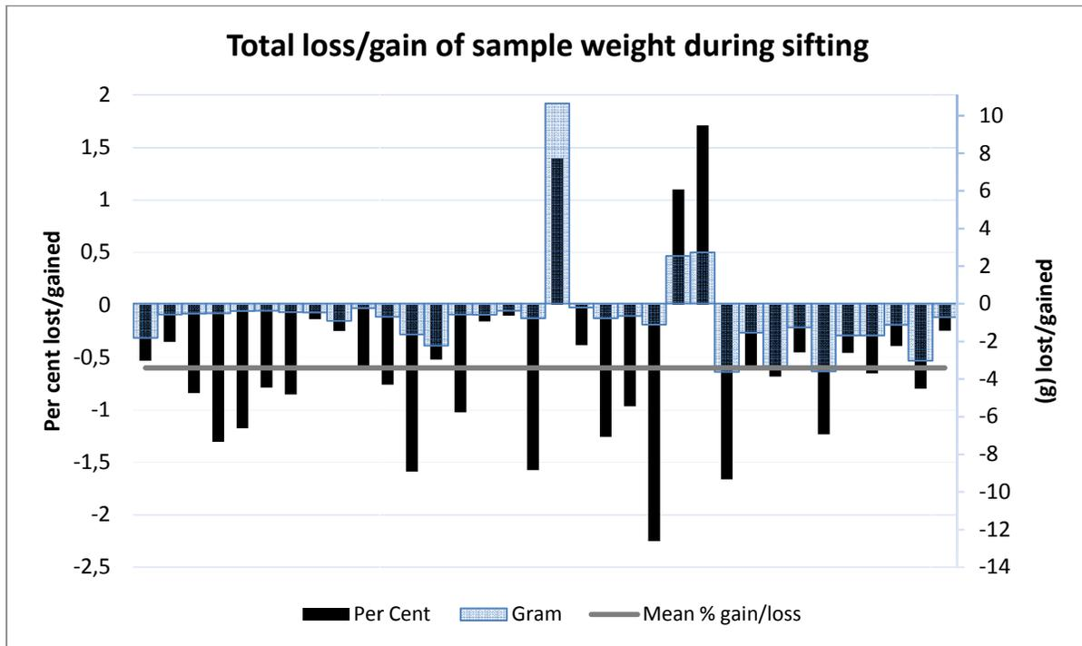
Figure 1: Per cent difference in total sample mass before and after sifting. The line indicates a general loss of 0,6 % of total sample weight. Samples presented here are from both Kvadehukun and Fuglehuken.
