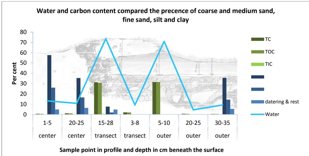
Figure 7: Per cent content of carbon and water related to particle size distribution in soil samples taken from the sorted circle. Grain sizes are grouped into coarse and medium sand (1-0,126 mm), fine sand (0,125-0,064 mm), and silt and clay (smaller than 0,063 mm). The sequence shows (from left) the fine grained center, the coarse border and the area outside the circle.
