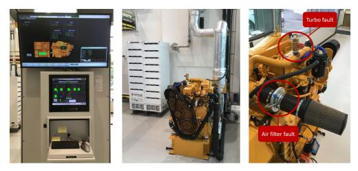
Figure 2.6: The hybrid power lab. The picture to the left shows the automation system, the picture in the middle shows the battery system and the diesel engine, while the picture to the right shows restriction devices used to provoke fault-types [5].
