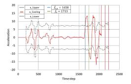
Figure 5.2: Online fault detection where p = 60 and the acceleration is used as the fault predictor for cooling degradation data [5].
