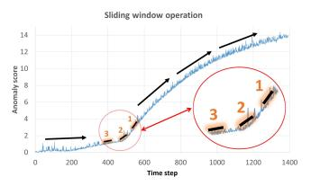
Figure 4.1: Illustration of the sliding window operation. Three windows (highlighted in orange) slide across AS through time [19].
