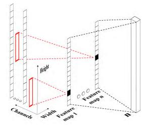
FIGURE 2. An illustration of the 1D convolution operation for multivariate time series data. The red rectangles represent 1D kernels.
