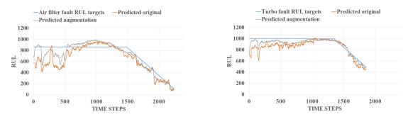
Fig. 9. The prediction results on the air filter fault and the turbo fault in the test set when the SkipRnet is trained on 20 augmented data sets and the original training set.
