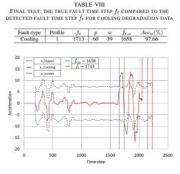
Fig. 7. Automatic fault detection where p = 60 and the acceleration is used as the fault detector for cooling degradation data.
