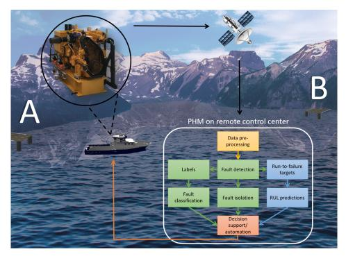
Figure 2.2: An autonomous ferry, crossing a fjord from dock A to B. The resulting analysis obtained from the data-driven PHM system can be used to schedule maintenance operations to the next appropriate dock of call.
