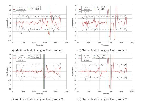
Figure 5.1: Online fault detection where p = 60 and the acceleration is used as the fault predictor for air filter and turbo degradation data [5].
