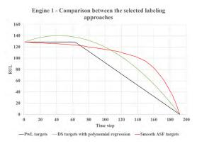
FIGURE 6. Comparison between the selected data-driven labeling approaches for engine 1.
