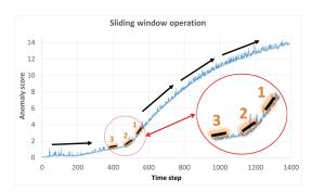
**FIGURE 4.** Illustration of the sliding window operation. Three windows (highlighted in orange) slide across *S*<sub>1</sub> through time.
