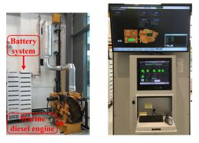
Fig. 2. The battery system, the marine diesel engine, and the automation system used for collecting the data sets.
