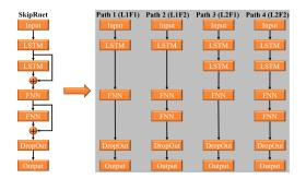
Fig. 1. The SkipRnet and its four different paths, L1F1, L1F2, L2F1, and L2F2, where L and F represent the number of LSTM layers and FNN layers, respectively.
