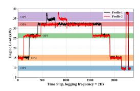
Fig. 3. Engine load profile 1 and 2.
