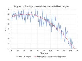
FIGURE 4. Comparison between raw DS targets and DS targets with polynomial regression for engine 1.
