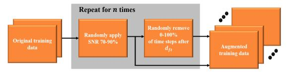
Fig. 4. The proposed data augmentation technique for run-to-failure time-series data.
