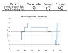
Fig. 2. Operating profile for a simulated autonomous ferry crossing.
