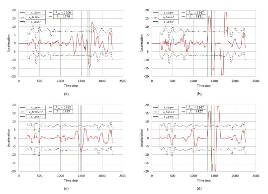
Fig. 6. Automatic fault detection where p = 60 and the acceleration is used as the fault detector. (a) Air filter fault in engine load profile 1. (b) Turbo fault in engine load profile 1. (c) Air filter fault in engine load profile 2. (d) Turbo fault in engine load profile 2.
