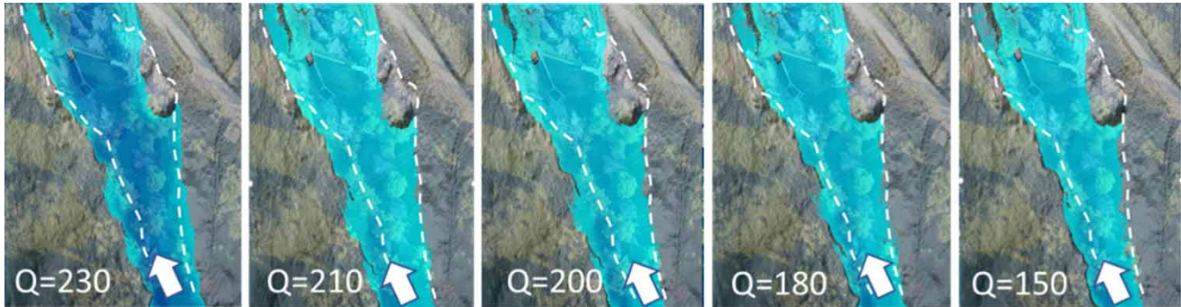
Figure 15 | Simulated water-covered area in Hec-Ras compared to areas with significant erosion observed.
