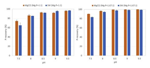
Fig. 2. The measured P-recovery in unseeded crystallization experiments with synthetic reject water by using seawater and MgCl<sub>2</sub> (adapted from Shaddel et al., 2020).
