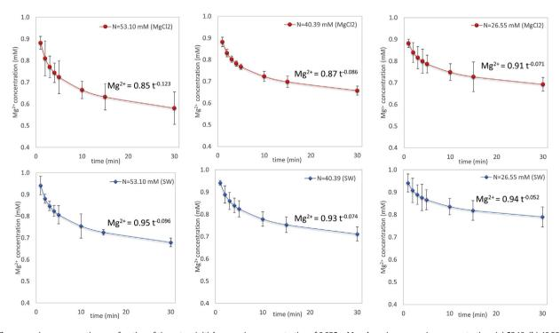
Fig. 3. The magnesium consumption as a function of time at an initial magnesium concentration of 0.925 mM and varying ammonium concentrations (a) 53.10, (b) 40.39, and (c) 26.55 mM with using MgCl<sub>2</sub> or seawater (SW) as the magnesium source.
