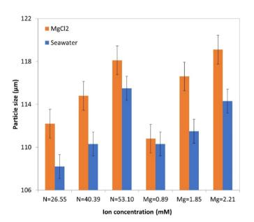
Fig. 6. The median size of particles after 60 min growth experiments (Seed  $_{median}$   $_{size}$  = 106.2  $\mu m$ ).
