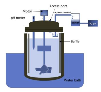
Fig. 1. The schematic representation of the reactor setup.
