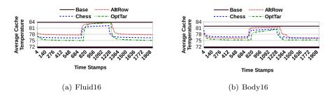
Fig. 17. Snapshot of temporal changes in average temperature of L2 during execution.
