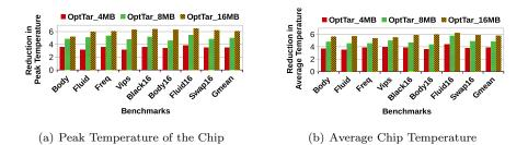
Fig. 23. Comparing temperature reduction (in  $^{\circ}C$ ) with different cache sizes.
