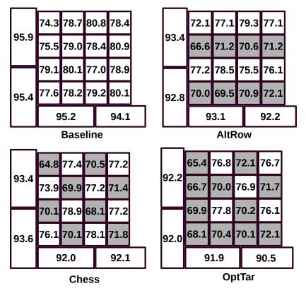
Fig. 19. Temperatures (in  $^{\circ}$ C) of the individual banks during **r**, for Fluid16.
