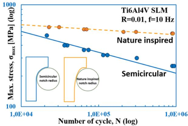
Figure 2: Fatigue results and comparison between a constant notch radius and a nature-inspired radius
