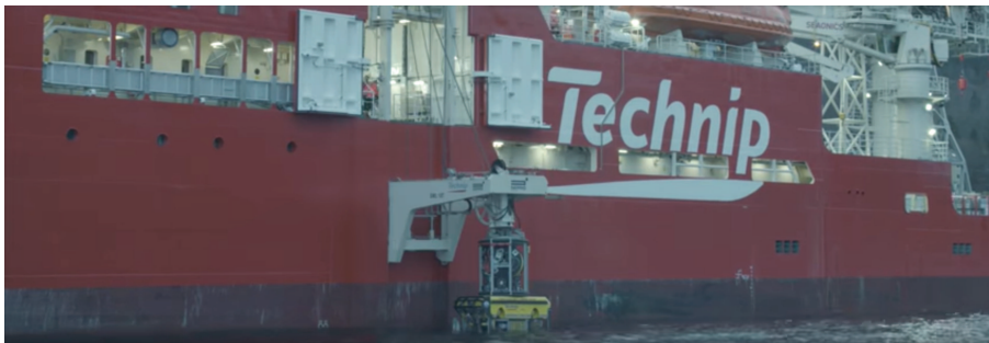
(a) Object lowered off to the side of the vessel, an alternative to lowering an object through the moonpool ( https://www.youtube.com/watch?v=wYcS6shEUwo )
