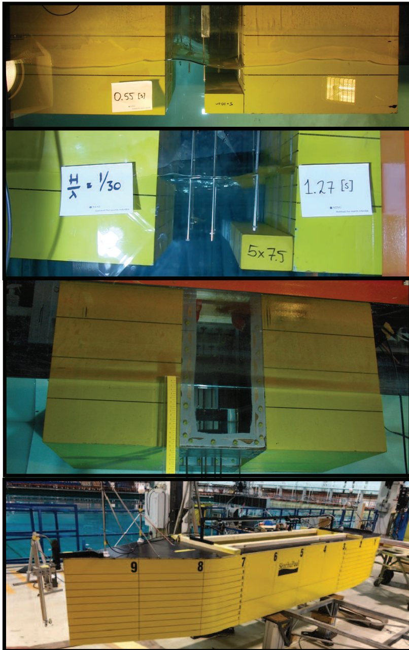
Figure 1.3: Photos of models with moonpools from the present model tests. The model tests are performed in two-dimensional and three-dimensional settings.
