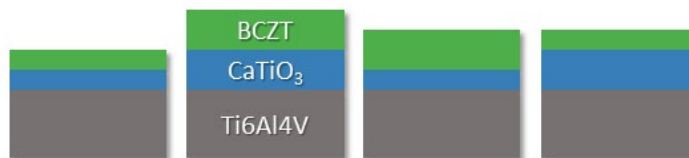
Figure 7.15: Schematic of the bi-layer ceramic coating thicknesses on Ti6Al4V. Combinations of thin and thick ceramic coatings were achieved by deposition of 20 or 40 layers of \text{CaTiO}_3 and BCZT slurries.
