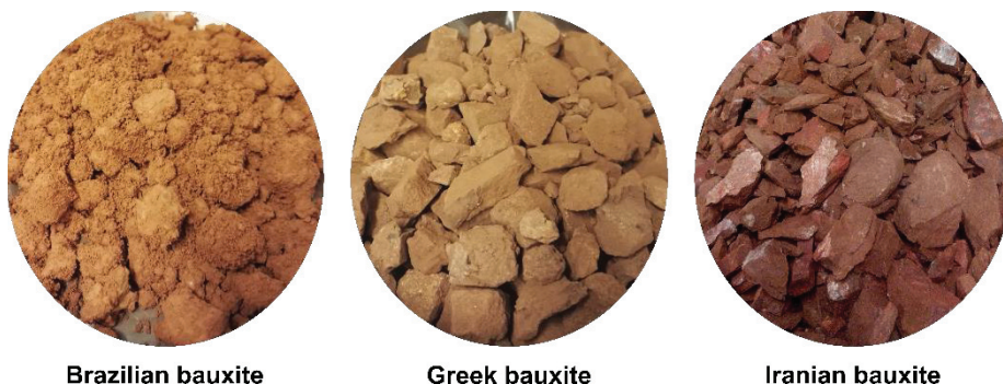
Fig. 3.7 Brazilian, Greek, and Iranian low-grade bauxites used in the study.
