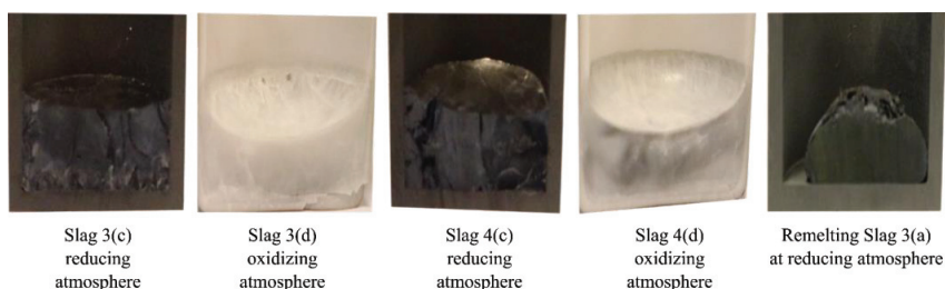
Fig. 4. A cross-section view of Slags 3(c), 3(d), 4(c), 4(d), and the remelted Slag 3(a).
