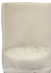
Slag produced in an oxidizing atmosphere (alumina crucible)
