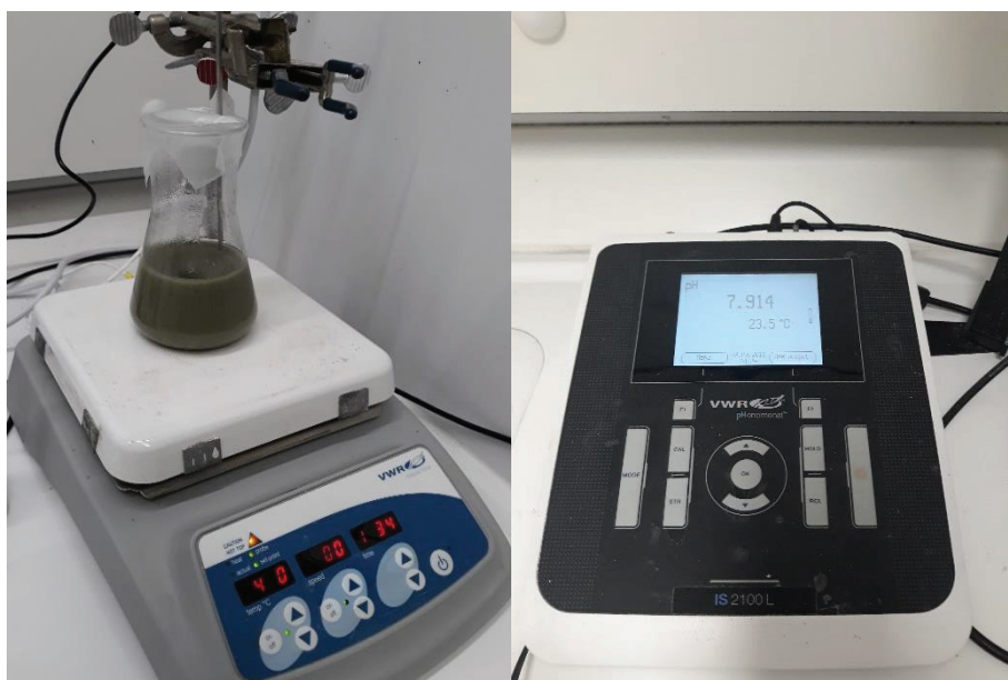
Fig. 4.1 Leaching experiment using a hot plate, beaker glass, and pH meter. pH meter was used to measure pH value continuously during the leaching trials.
