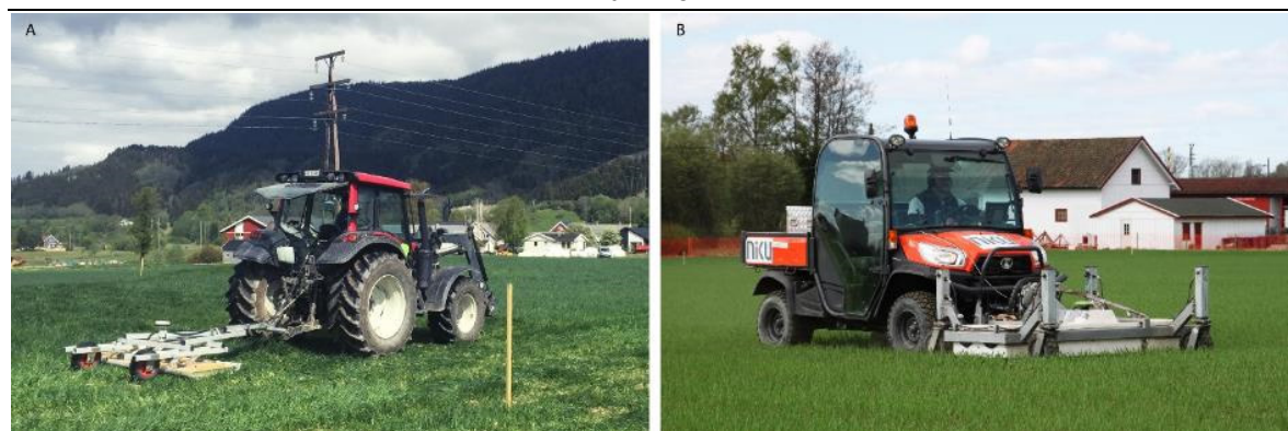
Figure 4. A. 3D Radar Mk IV Geoscope collecting data at Øya. B. MALÅ MIRA III in use at Dilling.
