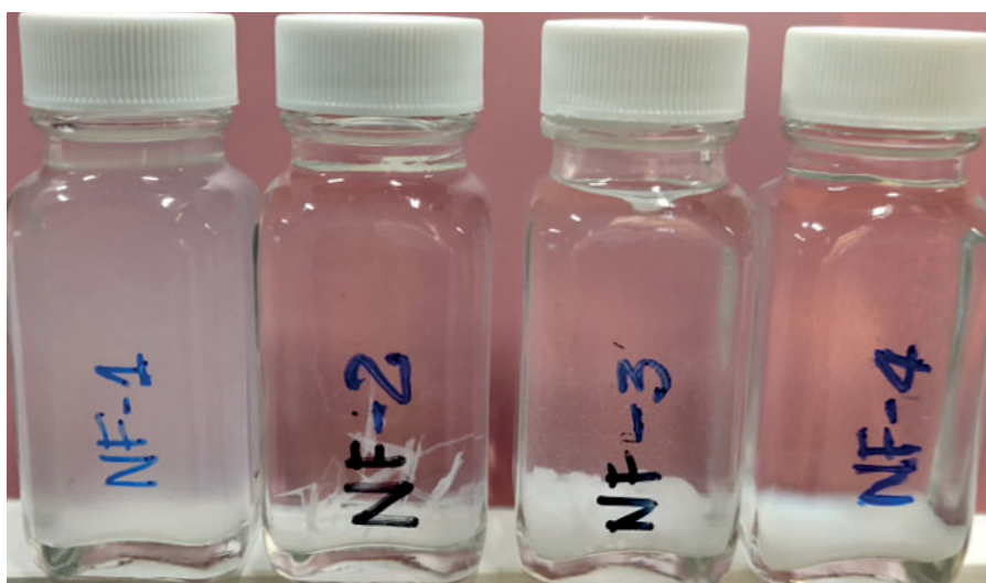
Figure 5.1: Visual analysis of NPs' stability in SSW at 60 °C. The white colour shows aggregated NPs. From left to right, labels refer to NF02-3, NF02-4, NF02-6 and NF02-8, respectively.
