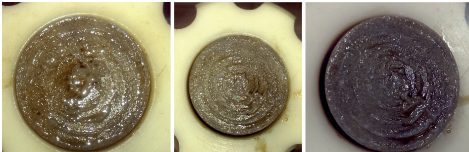
Figure 5.19: Filter cake build-up at core inlet during the nanofluid (NF02-6 and NF02-8) injection.
