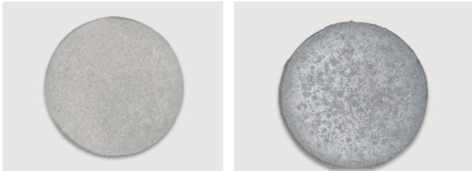
Figure 5.1.6: Images of ALD (a) and sputter (b) coated polished samples after 24 hours of immersion in SBF
