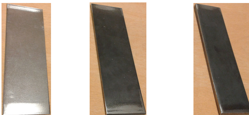
Figure 4.1 Specimens of the tank steels with thicknesses of 1.25 mm (Left), 4 mm (Middle) and 6 mm (Right)
