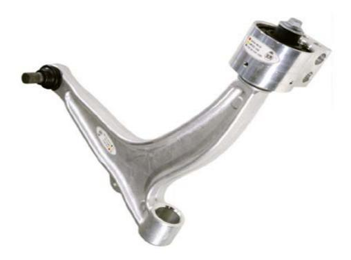
Figure 9.1: Front Suspension arm.
