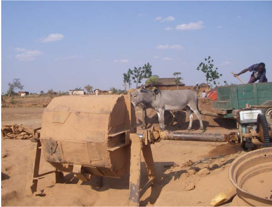
Fig. 5. 4 Crusher at crushing site. The material is brought to site by donkeys.
