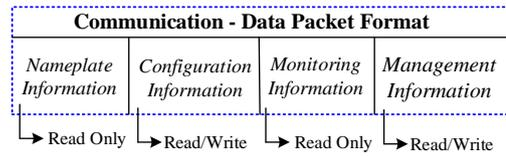
Fig. 3. Data packet configuration proposed in [15].
