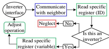
Fig. 4. Example of communication through SunSpec protocol in a general consensus-based cooperative strategy.
