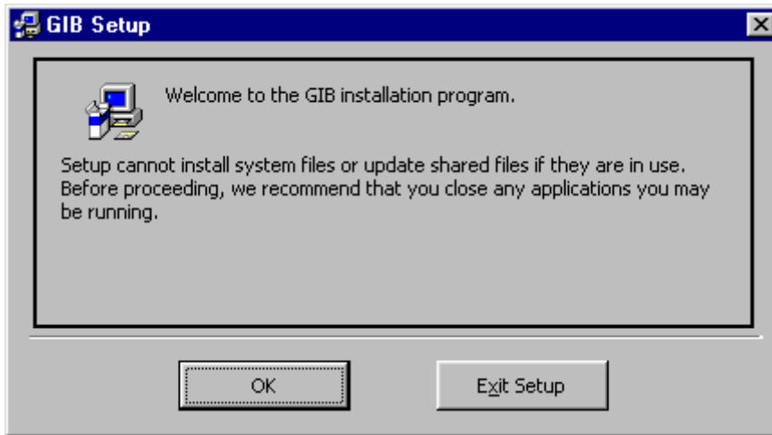
Figure 1.3.2 After launching the installation program, you are welcomed. It is recommended to close all other running programs before running the setup.
