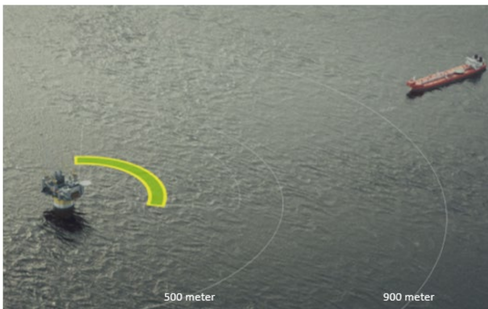
Figure 1 An overview of the stepwise sequence where a shuttle tanker approaches an offloading unit to start offloading oil to the ship (copyright: Kongsberg Group).
