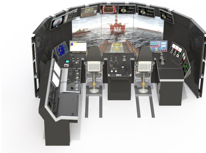
Figure 2 Layout of a bridge simulator (copyright: Kongsberg Group).
