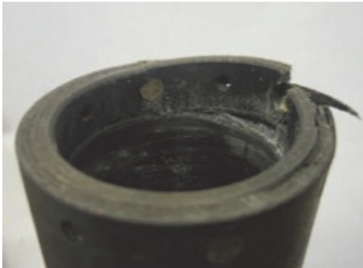
Figure 4.6 – Actuation ball ejected through seat of flow tube 4.40
