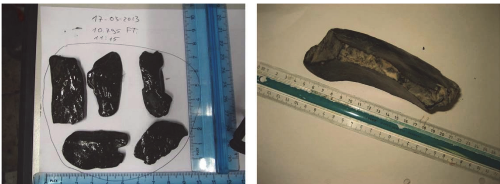
Figure E.1 – Pictures of cavings (van Oort et al. 2019, Fig. 1)
