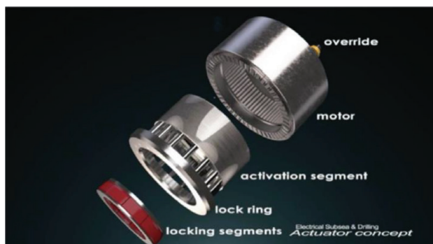
Figure 2. Electro-mechanical ring piston concept by ESD. The rotary motion of the electric motor is transmitted to the linear motion of the activation segment. Hydraulic modules can be removed with this design concept (Dale, 2013).
