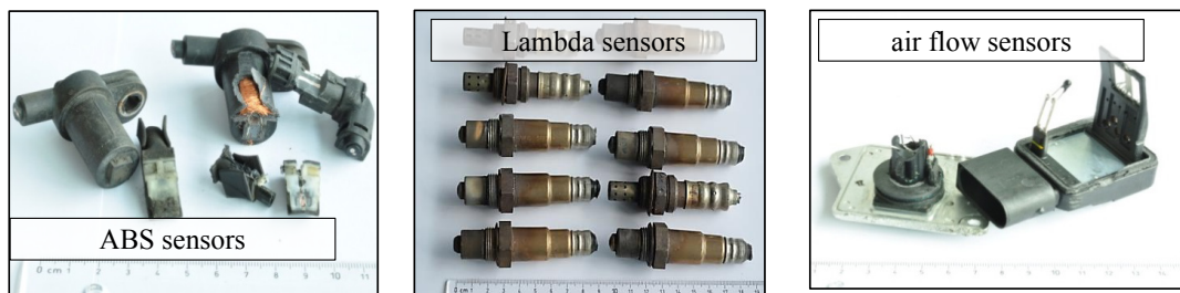
Figure SI 6: Photos of sampled EE components: ABS sensor's plastic and metal part, sensor element in lambda probe (removed in picture) and resistor from air mass flow meters.
