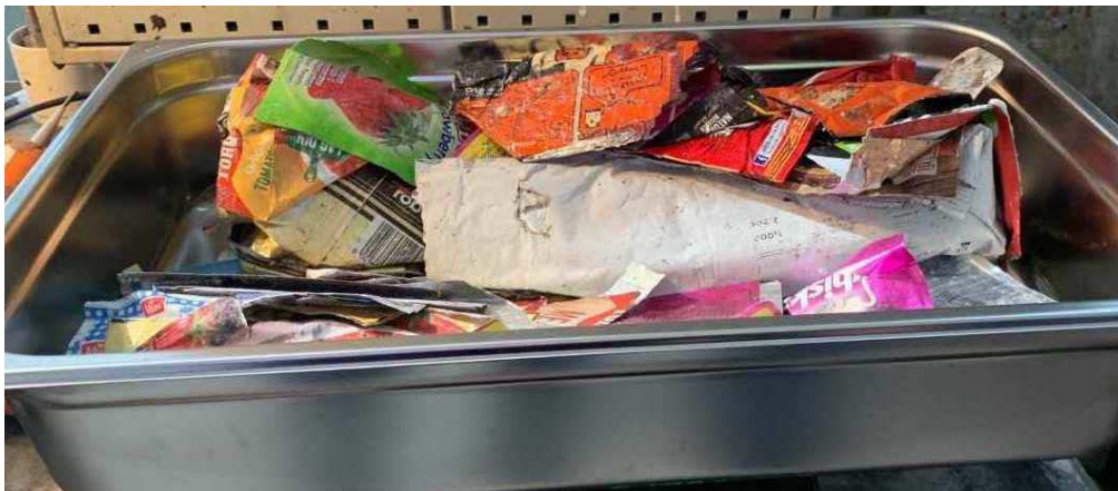
Figure 1: The Foils sample material, composed of thin laminates with aluminium, lacquer and plastics.
